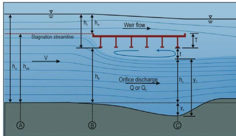
Figure 6.18. Vertical contraction and definition for geometric parameters.
