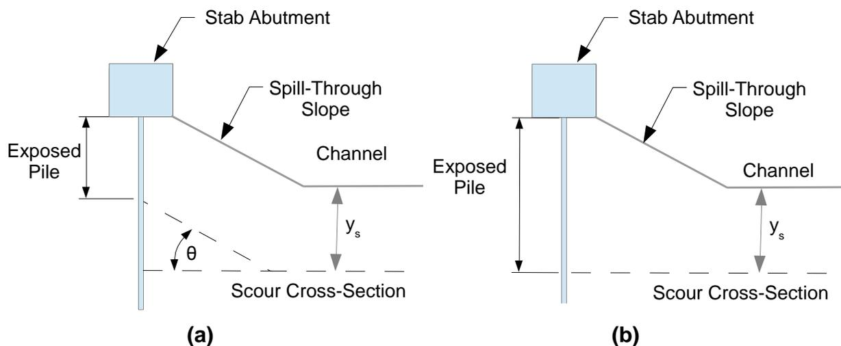
$y_s$  = sum of contraction scour, degradation and effect of lateral channel movement.
