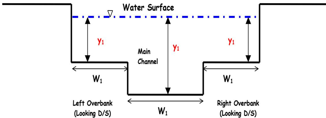
**Figure 1-2: Definition sketch for the Approach Section (Looking Downstream)**
