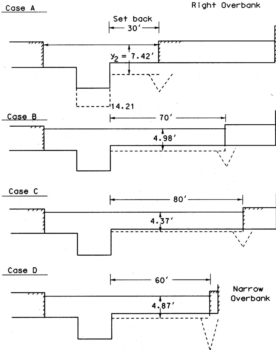
Figure A1-2: Scour Profile of Right Overbank for Different Abutment Setbacks
