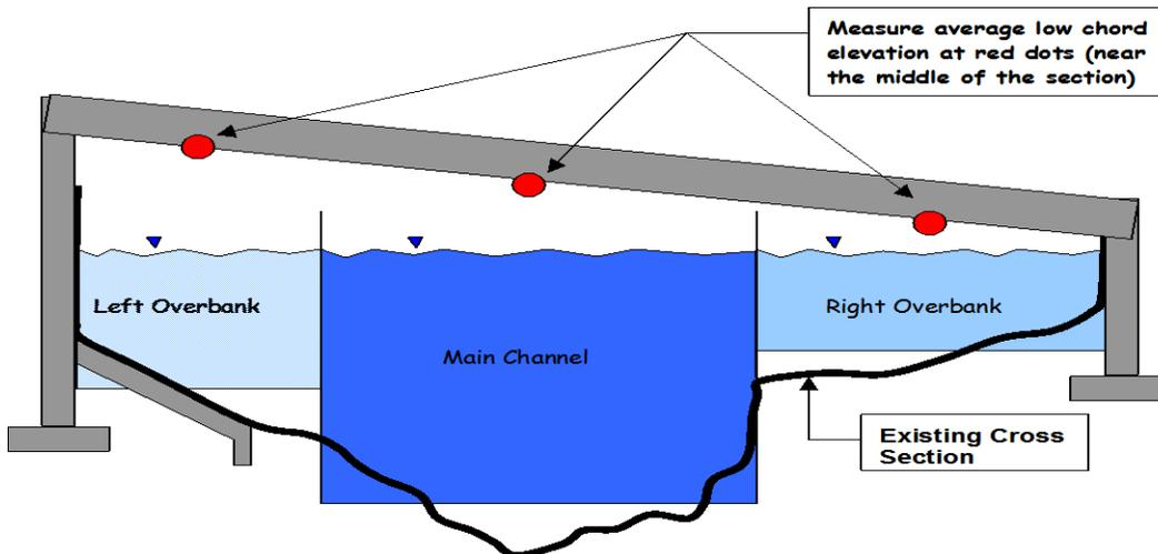
**Figure 2-11: Input Values for Low Chord Elevations**
