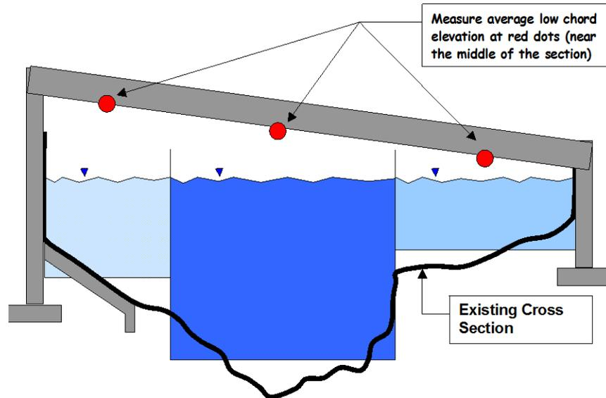
**Figure 2-8: Average Low Chord Elevation**
