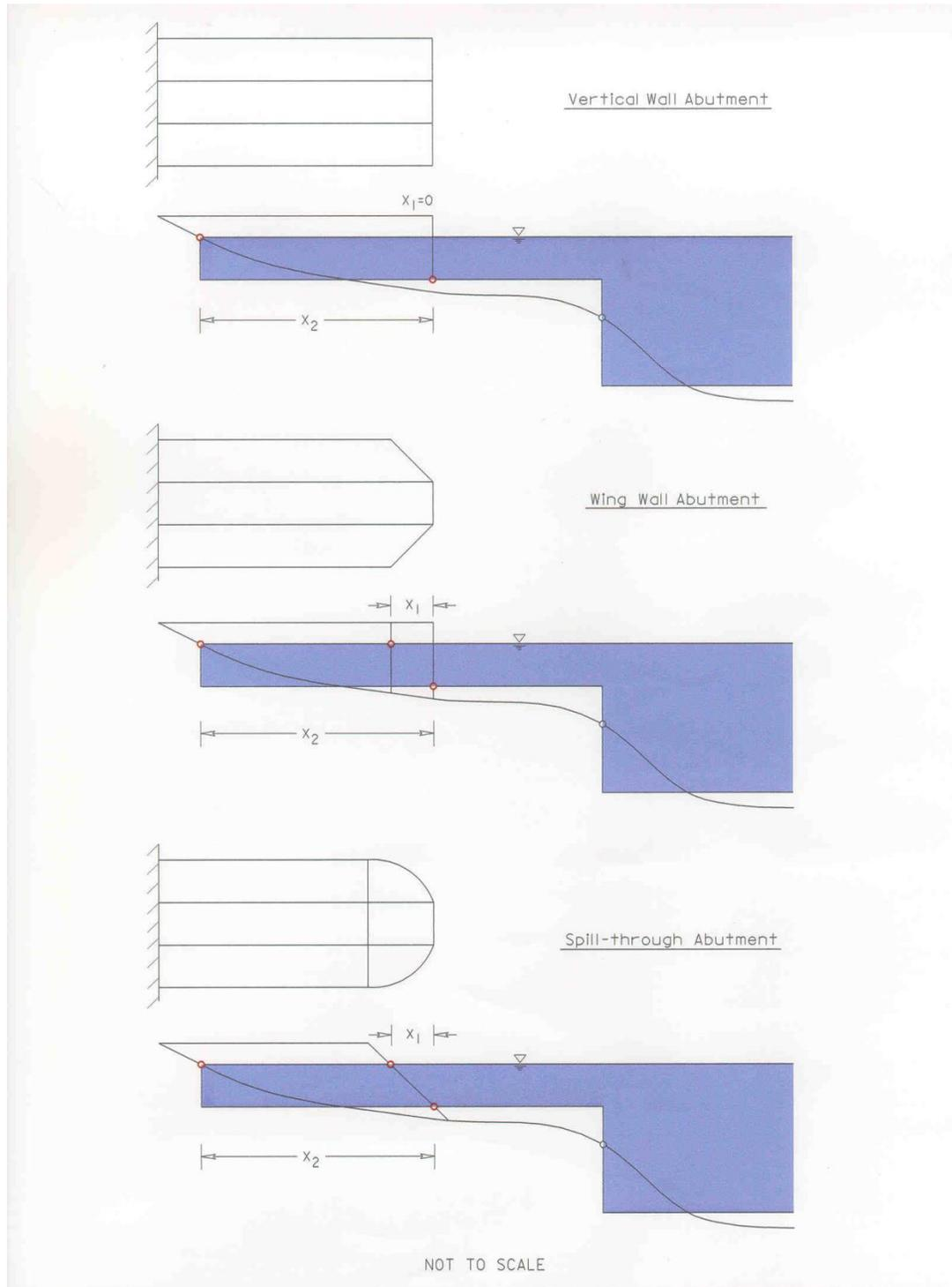
Figure 2-12 Abutment Shape Factor
