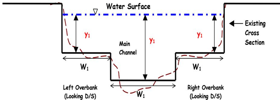
Figure 2-3: Definition Sketch for ABSCOUR Approach Section (Looking Downstream)
