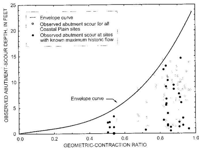
**Figure 76.** Relation of observed clear-water abutment-scour depth and the 100-year-flow geometric-contraction ratio identifying sites with known maximum historic flows in the Coastal Plain of South Carolina.
