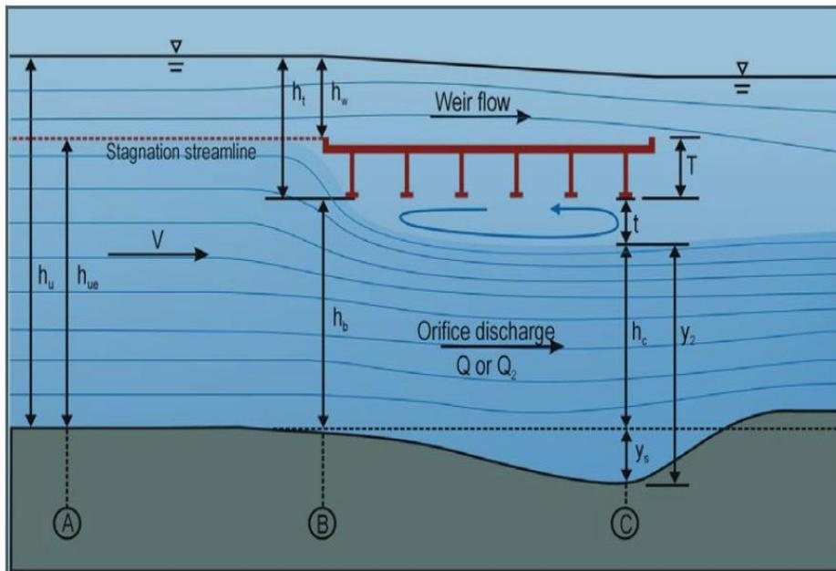
Figure 1-6 Definition Sketch for Upstream Bridge Data
