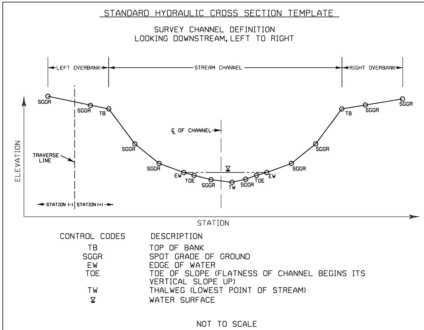
**Figure 5-6. Survey Data Requirements for Cross Sections**
