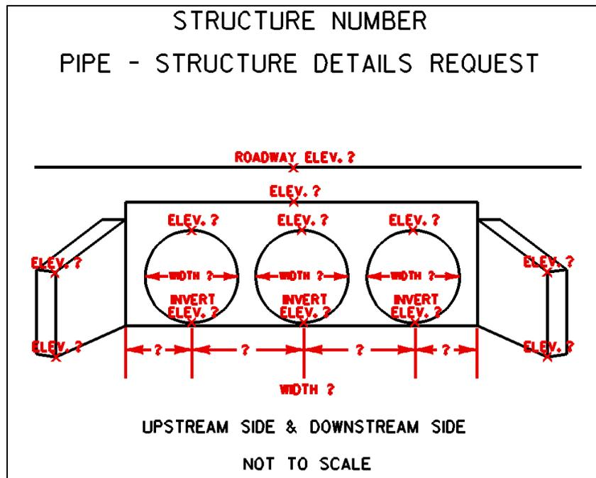
Figure 5-7. Survey Data Requirements for Pipe Structures
