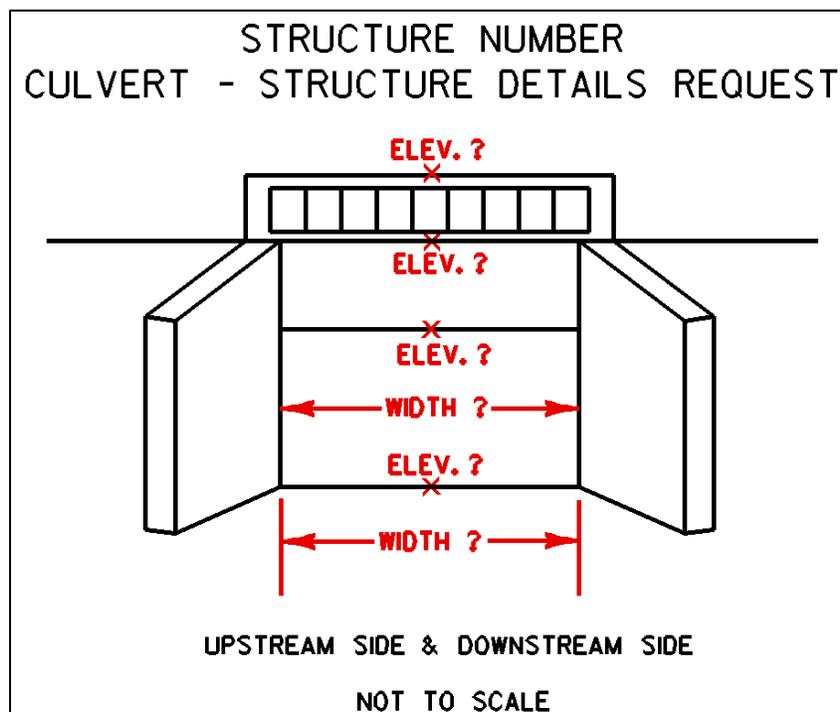
Figure 5-8. Survey Data Requirements for Culvert Structures
