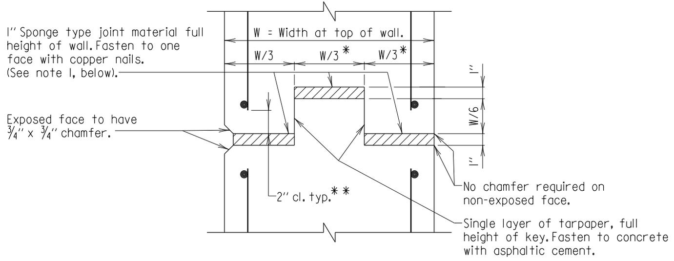
1" Sponge type joint material full height of wall. Fasten to one face with copper nails. (See note 1, below).
