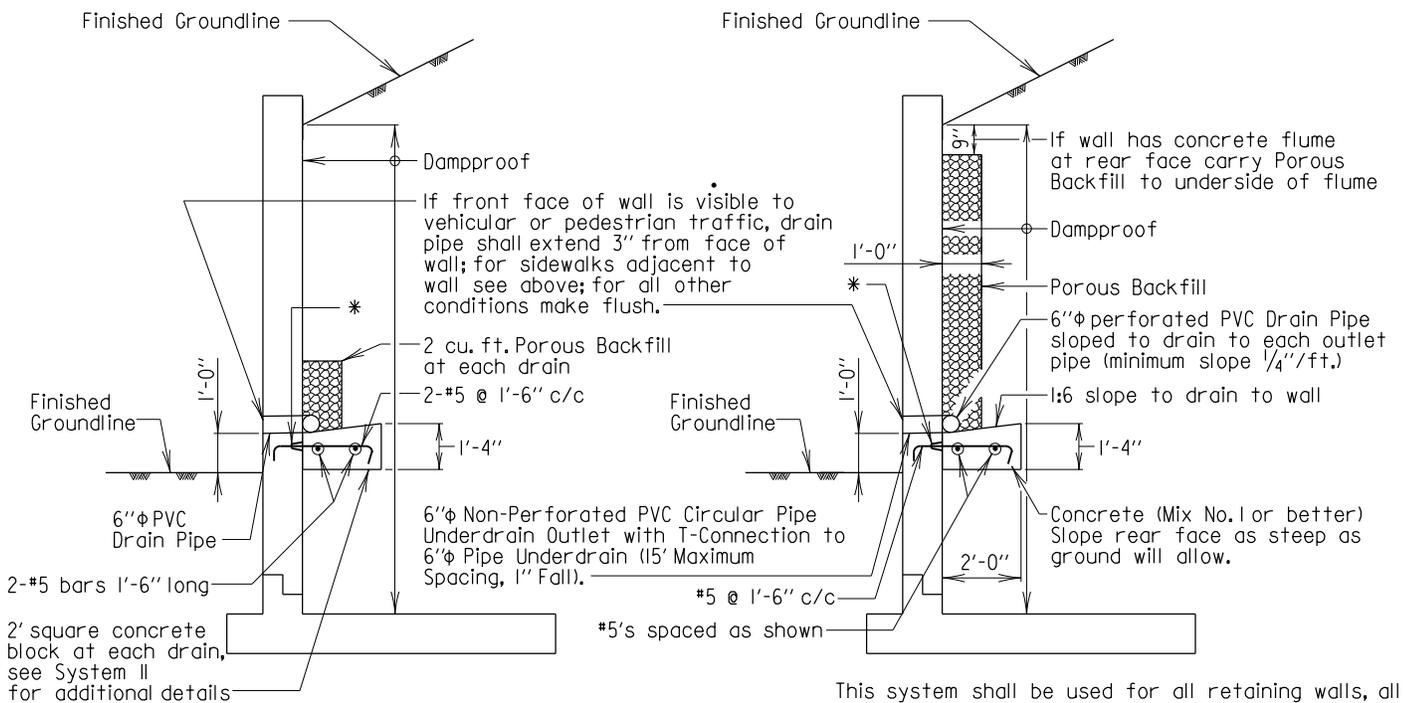
This system shall be used for all box culvert wing walls and other wing walls that are both less than 30' long and less than 16' high (height of wall from bottom of footing to top of highest section). One drain shall be placed at C of wall for all walls less than 15' long. For walls between 15' and 30' long, two drains shall be placed, one at each third point.
