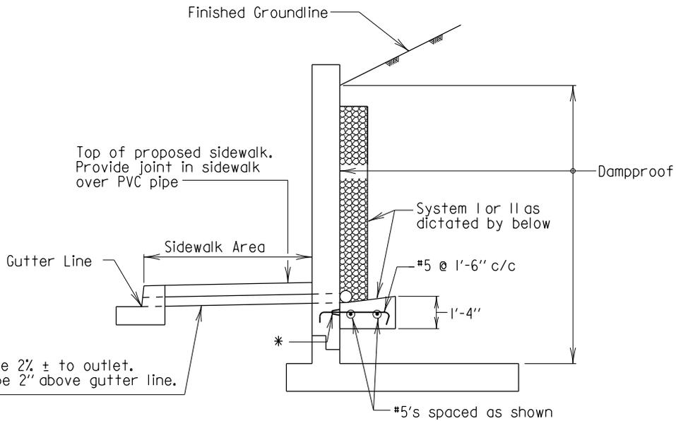
4"φ PVC pipe. Slope pipe 2% ± to outlet. Invert at outlet to be 2" above gutter line. (15' Maximum Spacing)
