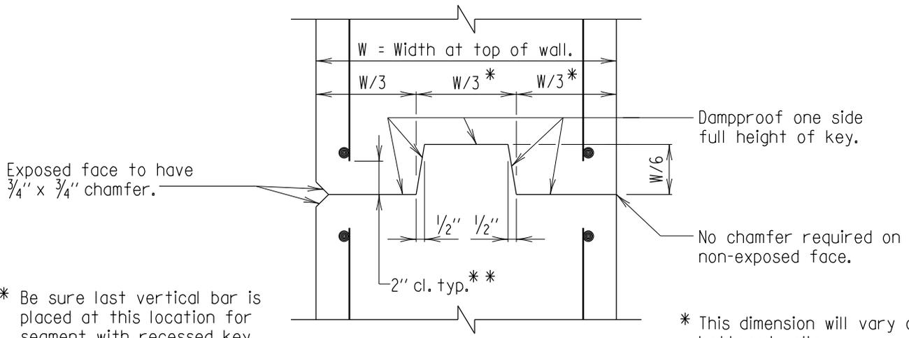
\*\* Be sure last vertical bar is placed at this location for segment with recessed key.
