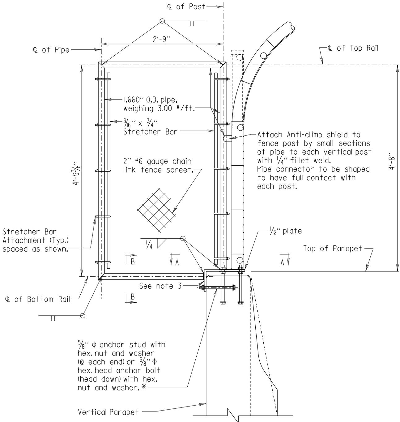
Stretcher Bar Attachment (Typ.) spaced as shown.
