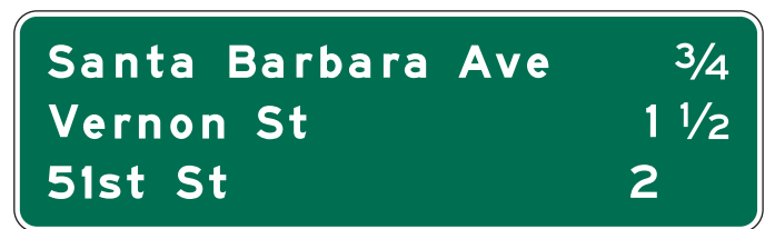
Figure 2E-31. Interchange Sequence Sign
