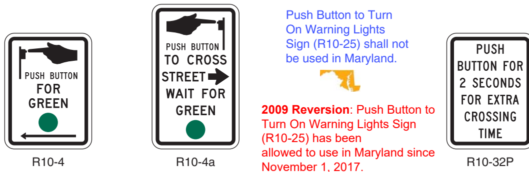
Figure 2B-26. Pedestrian Signs and Plaques (Sheet 2 of 2)
