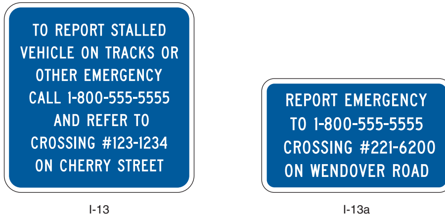
Figure 8B-4. Emergency Notification Signs
