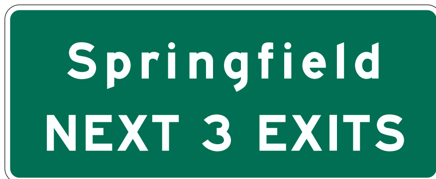
Figure 2E-26. NEXT EXITS Sign
