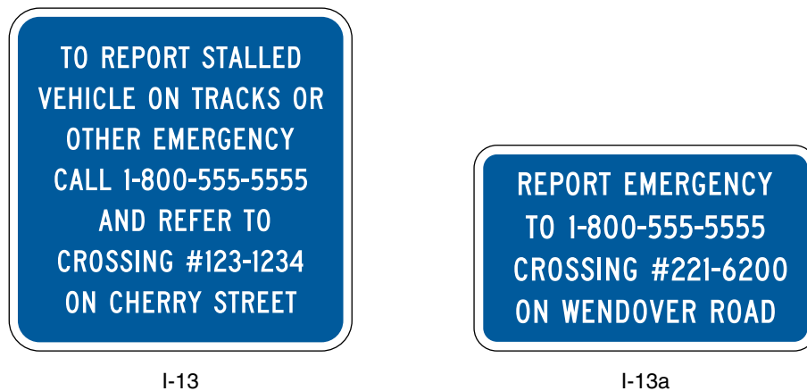
Figure 10C-4. Emergency Notification Signs
