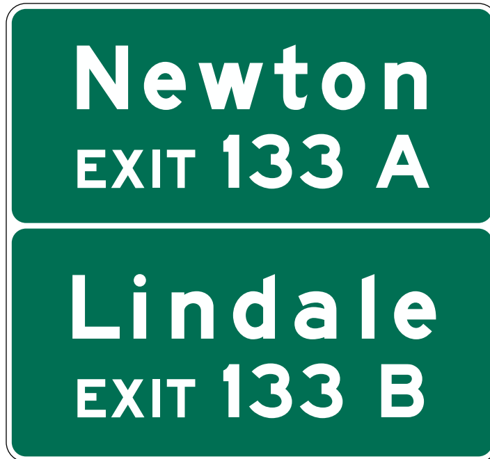
Figure 2E-17. Supplemental Guide Signs for Multi-exit Interchanges
