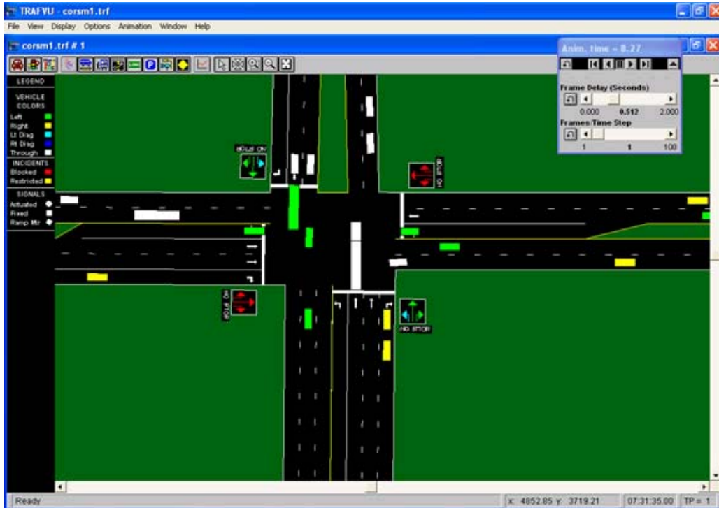
Figure 4.3: An actuated controlled signal designed with CORSIM.
