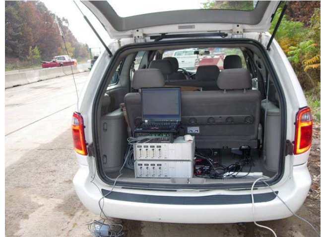
Figure 5.8 – ATI Wireless Data acquisition system for data processing
