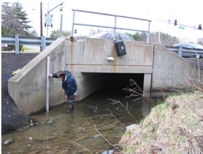
Figure 2.2: Continuous water level meter at upstream monitoring site
